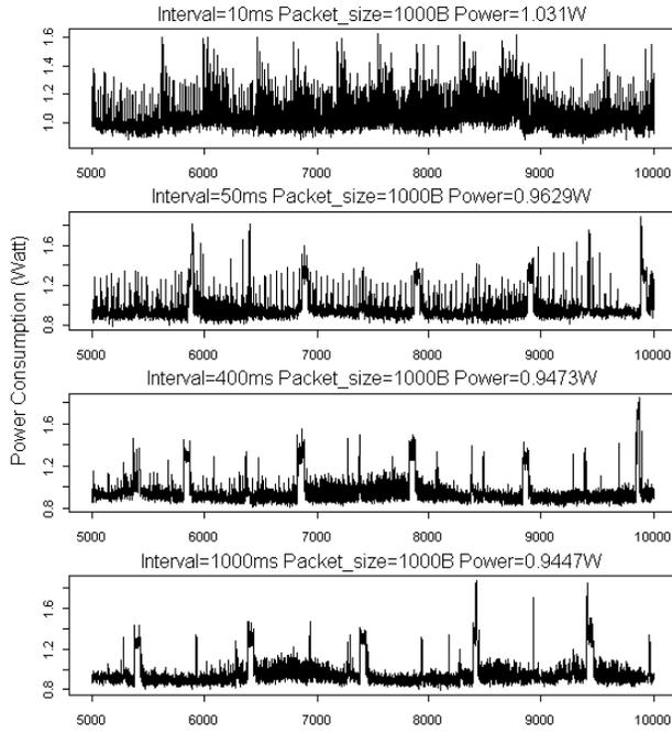
Fig. 1. Power Consumption of N900 in Downlink
