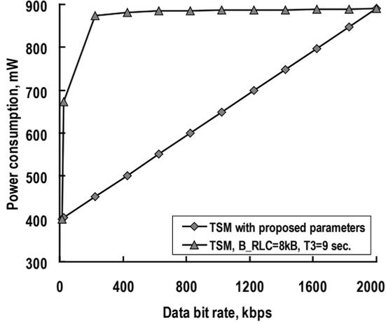
Fig. 4. Uplink power consumption for transition state machine for constant bit rate data transmission,  $c_2 = 16$  kbps,  $c_3 = 2000$  kbps,  $p_2 = 400$  mW,  $p_3 = 890$  mW
