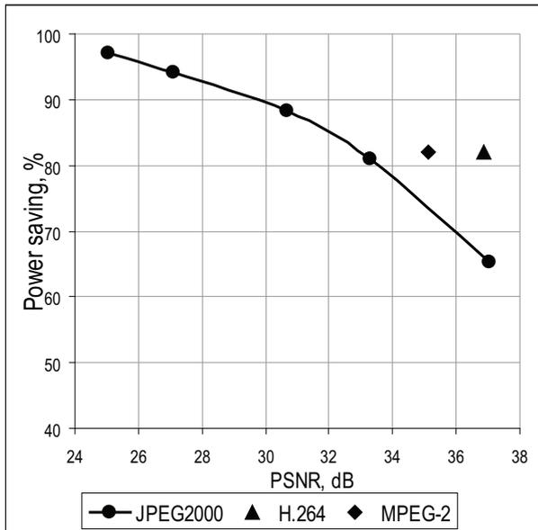
Figure 7: Relation between average PSNR and power saving for test video sequence “phenomenon“,  $B_b = 3\text{Mbps}$ .
