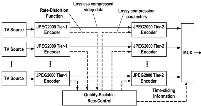
Figure 4: DVB-H Transmitter scheme based on JPEG2000 Encoder
