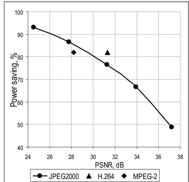
Figure 6: Relation between average PSNR and power saving for test video sequence "matrix",  $B_b = 3$ Mbps.
