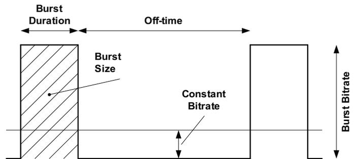
Figure 2: Time slicing in DVB-H [10]
