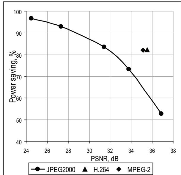
Figure 8: Relation between average PSNR and power saving for test video sequence “robin“,  $B_b = 3\text{Mbps}$ .
